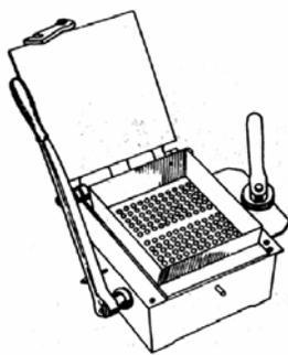
**Figure 2: Hand operated hard gelatin capsule filling machine**
