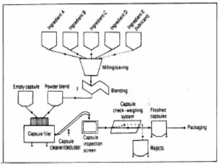
**Figure 3: Process flow diagram for automated capsule filling**
