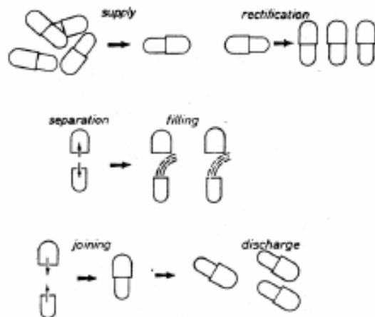
**Figure 4: The capsule filling process**
