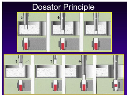
**Figure 5: Dosator principle of filling capsule**
