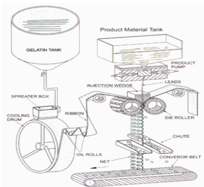
**Figure 8: Automatic Soft Gelatin Encapsulation Machine**
